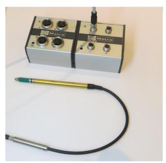
Measuring probes can be exchanged hot-plug. Means the sensor can be attached and dettached without a power down of the M-Bus.
